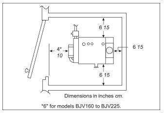
Figure 3. Closet and Alcove Installation (see Table 3).
